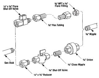
Figure 18. Supply valve connection fittings.
